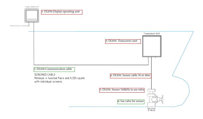
• The cable between Display unit (on the bridge) and transceiver unit (within 40m distance from the DL850 sensor) is a 4 pair cable with individual screen and a minimum size of 0.325mm.
